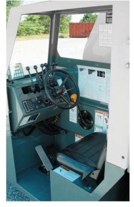
Standard:Open air cab shell w/overhead<br/>safety glassOptional:Closed cab with hinged door,<br/>heater, and defroster
