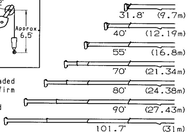
NOTE: Boom and jib geometry shown are for unloaded condition and machine standing level on firm supporting surface. Boom deflection and subsequent radius and boom angle change must be accounted for when applying load to hook.
