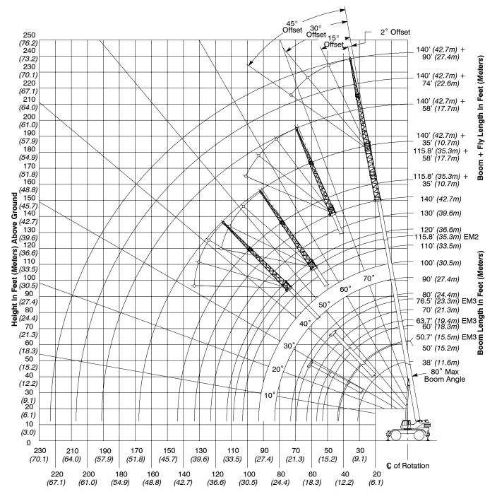
Operating Radius From Axis Of Rotation In Feet (Meters)
