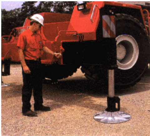
Fully Extended Outriggers 23' 0" (7.01 m) spread
