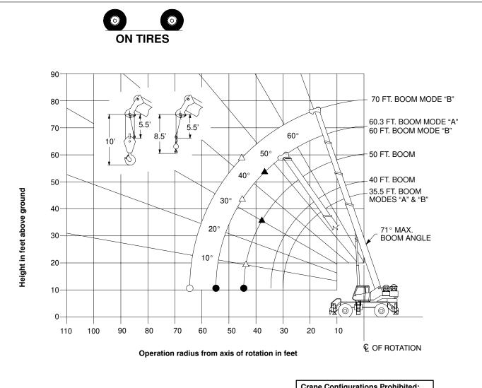
Crane Configurations Prohibited: Boom Lengths Greater than 71 FT. 28.5 FT. Offset Fly 51 FT. Offset Fly
