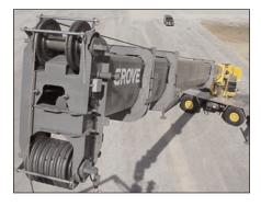
The 160 ft. (48.8 m) 5 section Full Power boom incorporates the "U" shaped MEGAFORM™ design, which eliminates stiffeners, thus reducing weight and increasing capacity.
