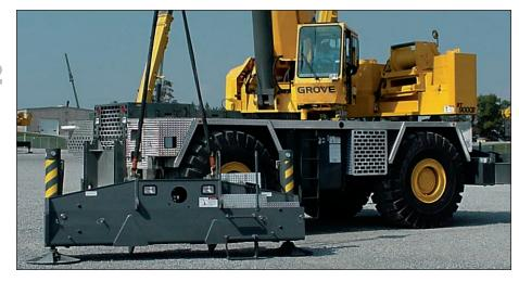
Removable front and rear outrigger boxes provide up to 19,374 lbs. (8 788 kg) of weight reduction for easier transport. Include the removable 40,000 lbs. (18 100 kg) of counterweight, auxiliary hoist and rope, and the RT9130E can easily self-remove close to 64,000 lbs. (29 000 kg).
