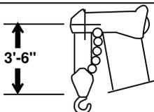
DIMENSIONS ARE FOR LARGEST GROVE FURNISHED HOOKBLOCK AND HEADACHE BALL, WITH ANTI-TWO BLOCK ACTIVATED.
