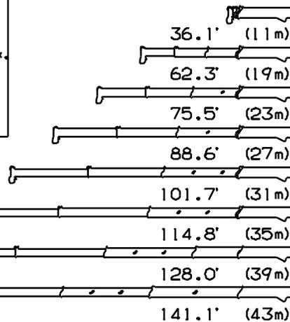
NOTE: 1. Boom and jib geometry shown are for unloaded condition and machine standing level on firm supporting surface. Boom deflection and subsequent radius and boom angle change must be accounted for when applying load to hook.
