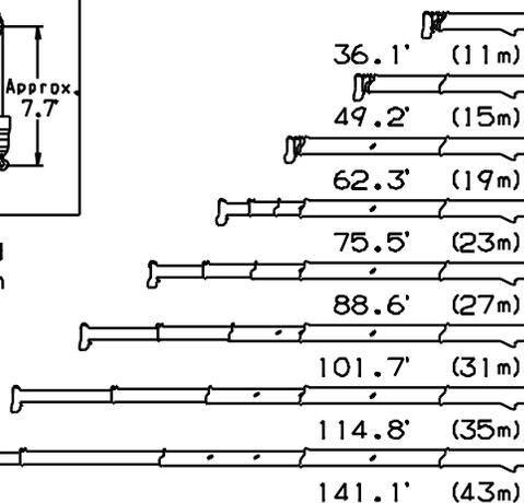
NOTE: 1. Boom and jib geometry shown are for unloaded condition and machine standing level on firm supporting surface. Boom deflection and subsequent radius and boom angle change must be accounted for when applying load to hook.
