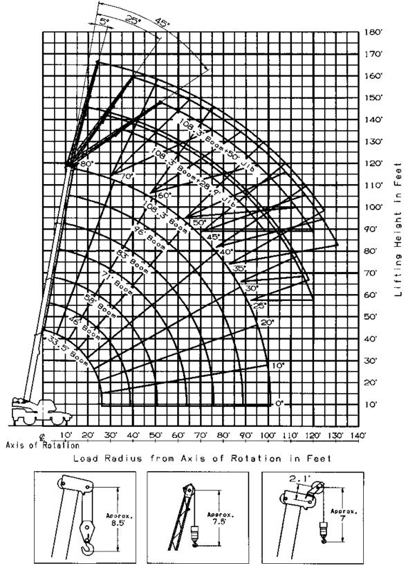
NOTE:Boom and jib geometry shown are for unloaded condition and machine standing level on firm supporting surface. Boom deflection and subsequent radius and boom angle change must be accounted for when applying load to hook.
