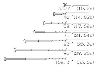
NOTE :Load radiuses for jib operation are given for reference with the boom fully extended to 108.3' (33m).
