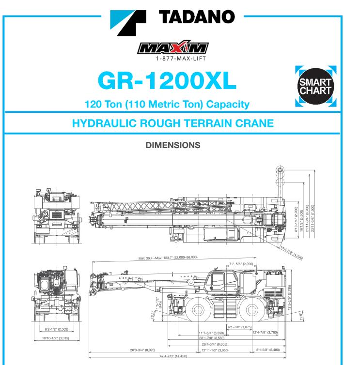
Note: Dimension is with boom angle at -1.5 degree. () Reference dimensions in mm.
