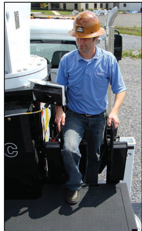
Walk Through Control Stations
