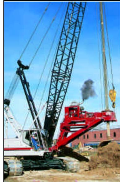
**Head machinery** includes standard lift crane sheaves with optional wide mouth sheaves available for duty cycle.
