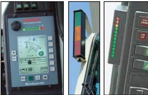
Integrated Microguard rated capacity limiter with color graphic display, for excellent contrast even in direct sunlight, aids the operator in safe and efficient operation by continuously monitoring a multitude of crane conditions. Optional external and internal light bars inform the operator and/or ground crew of the percentage of capacity.
