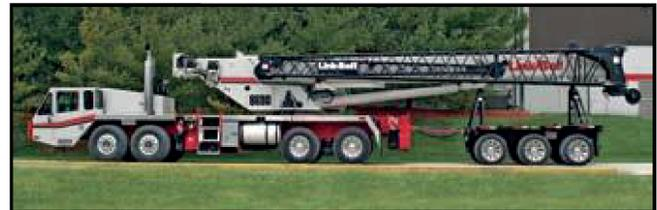
☐ Boom dolly/trailer ready when equipped with optional boom float kit and rear electrical and air connections
