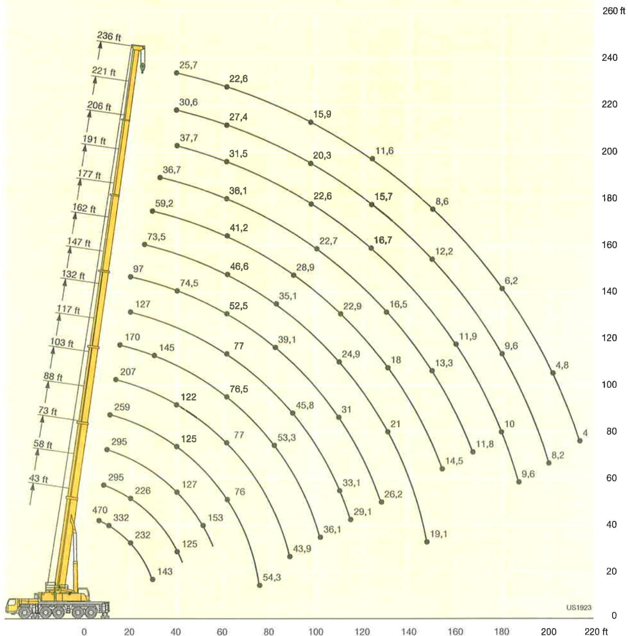
**Lifting capacities on the hydraulically or mechanically variable folding jib**
