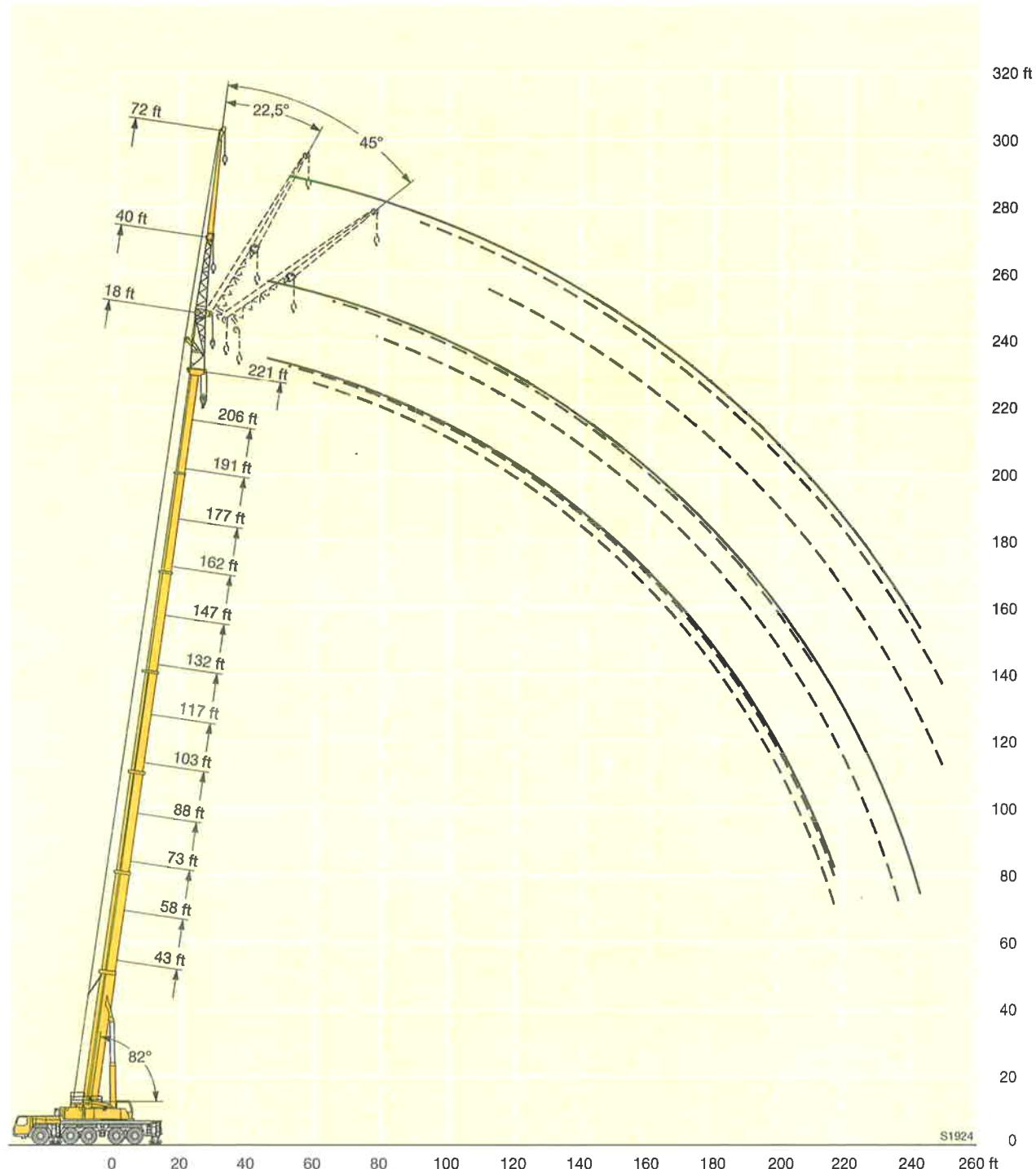
**Lifting capacities on the hydraulically or mechanically variable folding jib**
