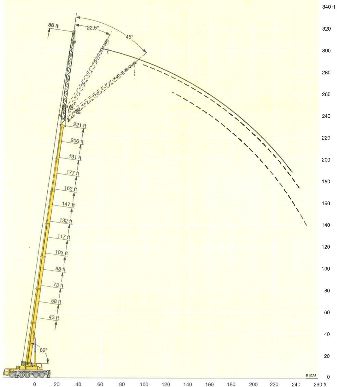
**Lifting capacities on the hydraulically or mechanically variable folding jib**
