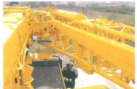
Hydraulic assembly assistance for attaching the folding jib
