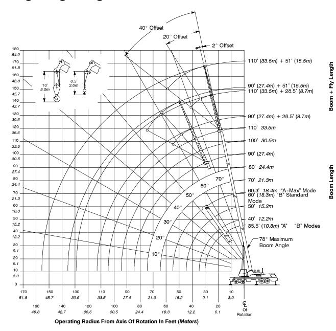
Note: Boom and fly geometry shown are for unloaded condition and crane standing level on firm supporting surface. Boom deflection subsequent radius and boom angle change must be accounted for when applying load to hook.
