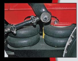
Raydan™ air-ride suspension front and rear provides a smooth ride and precise handling. Optional air-ride lift system holds the rear suspension retracted while the crane is on outriggers.
