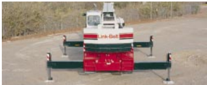
Fully Extended Outriggers 20' 6" (6.25 m) Spread
