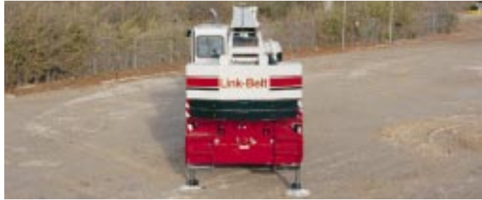
Retracted Outriggers 7' 9" (2.36 m) Spread
