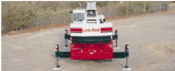
Intermediate Outriggers 14' 2" (4.32 m) Spread
