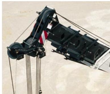
Basic boom extend mode – boom mode 'B'
