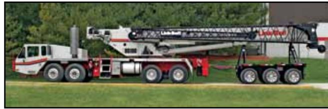
↑ Boom dolly/trailer ready when equipped with optional boom float kit and rear electrical and air connections
