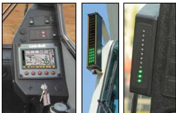
Link-Belt Pulse is the Link-Belt-designed total crane operating system. It includes the rated capacity limiter, extend mode controller, diagnostic capabilities, and continuous monitoring of multiple crane functions and conditions. To aid operators in safe and efficient operation, its high-resolution, color-intense graphic display provides excellent contrast even in direct sunlight.
