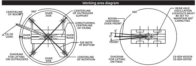
Bold lines determine the limiting position of any load for operation within working areas indicated.
