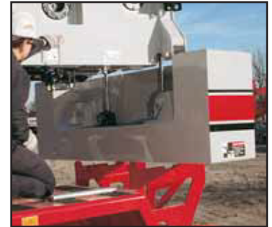
Fast & efficient hydraulic counterweight removal enhances roadability
