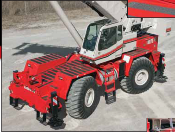
Fast & efficient hydraulic counterweight removal enhances roadability
