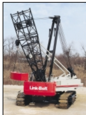
Optional 10' (3.05 m) boom extension handles treadmembers, counterweight and boom during self-stripdown or erection.
